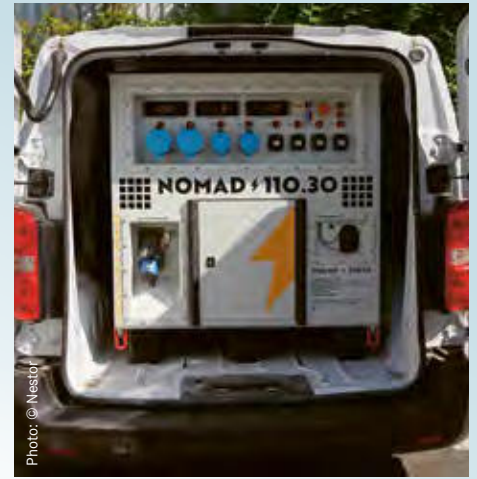
The Nomad110.30 offers a continuous output of 30 kVA
