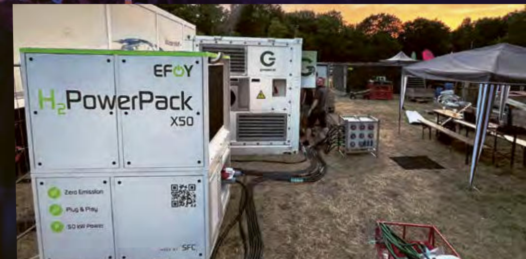
The 50 kW fuel cell generator provides the power supply for the main stage
