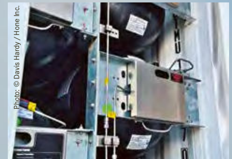
Trailer with eight tanks that contain 130 kg of hydrogen
